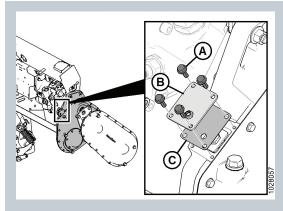
1. Remove four bolts (A), cover (B), and gasket (C) from the main gearbox.
