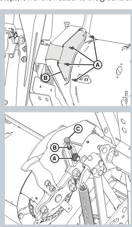
1. Remove four bolts (A) and inspection panel (B) to view chain.
