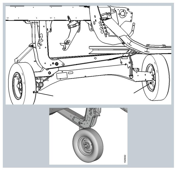
Lubricate wheel hubs, one zerk per wheel.
