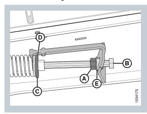
Adjust the draper tension by loosening jam nut (A) and turning bolt (B) clockwise to increase draper tension or counterclockwise to decrease draper tension.
