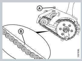
5. Turn adjuster thumbscrew (A) clockwise to increase tension until chain deflection (B) is 4 mm (0.16 in.) at midspan
