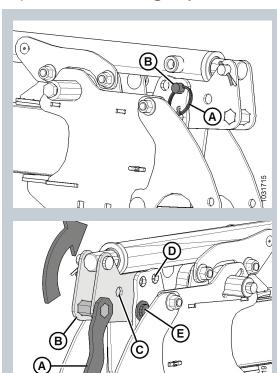
1. Remove split ring (A), clevis pin (B), and flat washer securing the right fore-aft cylinder in the forward position.
