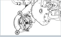
4. Remove three bolts (A) that secure input driveline guard base (B).
