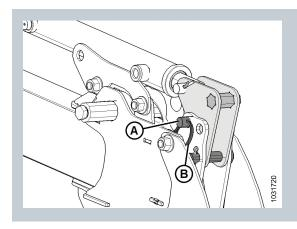
3. When the bracket holes are lined up, secure in aft position with clevis pin (A), washer, and split ring (B).
