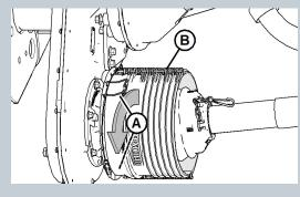
1. Pry clips (A) up to release shield (B).
