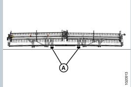
3. Place two 254 mm (10 in.) blocks (A) under the cutterbar, just inboard of the wing flex points.
