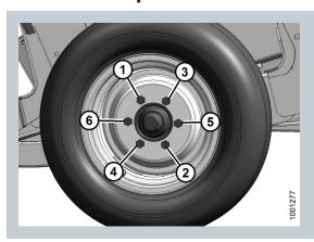
Follow the bolt tightening sequence shown and torque the wheel bolts to 110-120 Nm (80-90 lbf-ft).
