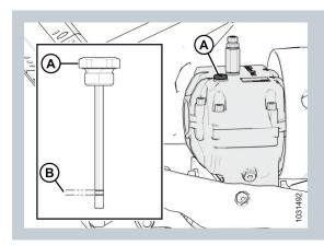
1. Remove oil level dipstick (A) and check the oil level. The oil level must be within range (B).
