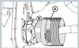
2. Slide shield (A) along driveline to access quick disconnect collar (B).
