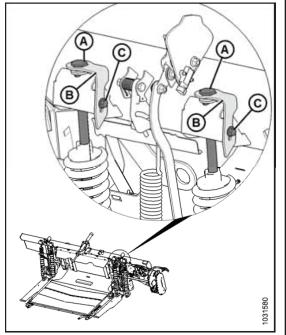
Figure 6: Float Adjustment Bolts - Left Side Shown
