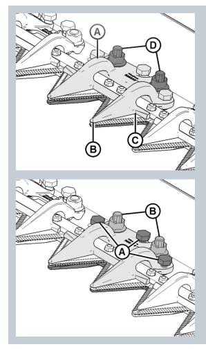
Manually stroke both knives to their inboard end so that knife sections are under hold-down (A).
