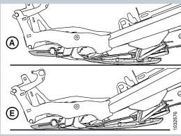
Shallowest angle (A) (center-link fully retracted) produces the highest stubble when cutting on the ground.
