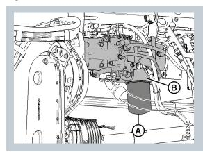
Change the oil filter after the first 50 hours of operation and every 250 hours thereafter.
