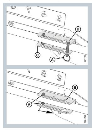
1. Remove split ring (A) and clevis pin (B) securing the left cylinder in forward position on cylinder bracket (C).
