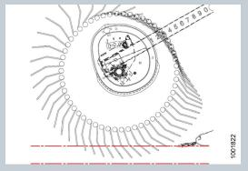
**Reel cam position 4** is for severely lodged crops where the reel will be placed in front of and possibly below the cutterbar. For best lifting action.
