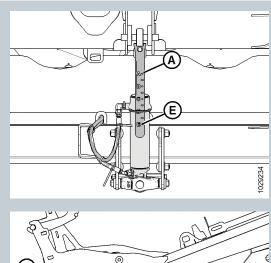
Use shallower settings (A) (position A on the indicator) for normal cutting conditions and wet soil to reduce soil buildup at the cutterbar. Shallow angle settings also minimize damage to the knife in stony fields.
