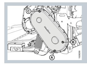
5. Add oil through filler plug (C) until it runs out of oil level hole
