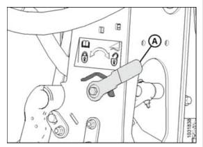
Figure 3: Float Unlocked - Left Side Shown
