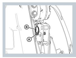
5. When the bracket holes are lined up, secure in aft position with clevis pin (A), washer, and split ring (B).
