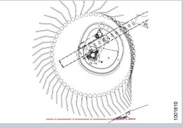
**Reel cam position 1** is recommended for straight cut canola where the reel will be pulled back behind the cutterbar and you want minimal reel finger engagement in the crop to limit loss.
