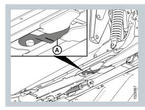
Before operation, ensure both link holder hooks (A) are engaged on the float module under the feed deck as shown. Inspect link holder hooks for any damage or wear. Replace if damaged/broken or missing.
