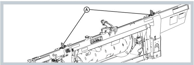
There are two float height sensors (A) installed on the float setting indicators on the float module. These sensors send signals to the combine allowing it to maintain a consistent cutting height and an optimum float as the header follows ground contours.
