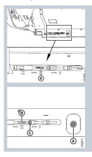
Ensure tensioner indicator (A) is approximately halfway in the window (covers the inboard half of the window).
