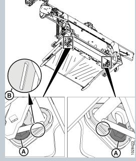
If bolt head (A) is closest to fixed symbol (B), the auger is in the fixed position.
